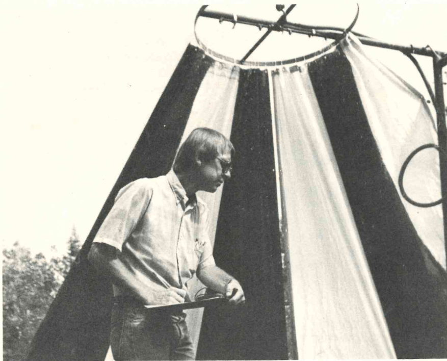
Tim Ward, an NMSU civil engineer, keeps track of runoff caused by simulated rainfall pouring from overhead sprinklers.
